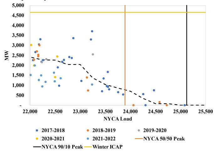
The dynamic limit shown here is calculated as median output at historical loads within 500 MW (systemwide) of each load level and is constrained to be strictly non-increasing.
