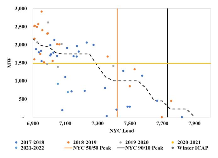
The dynamic limit shown here is calculated as median output at historical loads within and 100 MW of each load level and is constrained to be strictly non-increasing.
