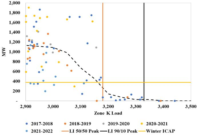
The dynamic limit shown here is calculated as median output at historical loads within and 100 MW of each load level and is constrained to be strictly non-increasing.
